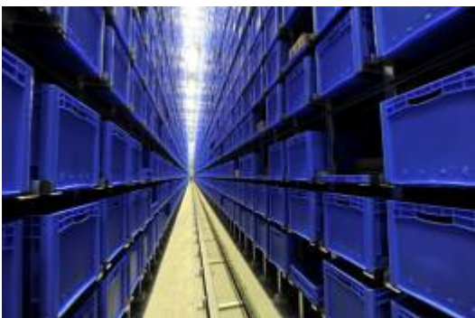
Picture 3: Incoming goods are packed into BITO containers of different sizes and then fed into the automated small parts storage facility for interim storage.
