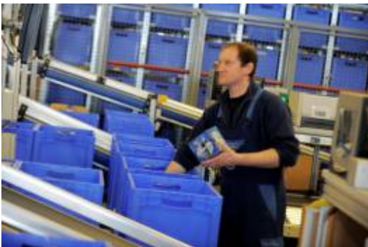
Picture 2: The BITO container system in European standard sizes which is employed in all logistic processes at Optimal allowed to accelerate material flow and increase order picking performance.
